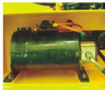
Side mounted hoist motor for easy maintenance
