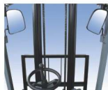
Wide view mast for clear front operator visibility
