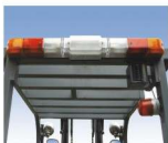
High Mounted Rear Combination and Beacon Lights
