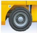
Minimum rear overhang for less turning radius
