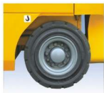
Minimum rear overhang for less turning radius
