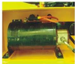
Rear Side mounted hoist motor for easy maintenance
